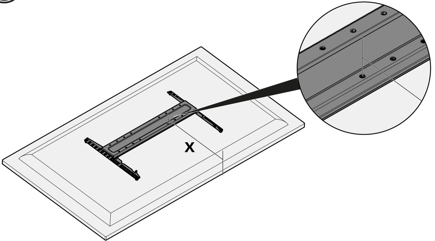
Place the Backplate in the top slot on the TV Brackets. Measure from the lower mounting holes on the Backplate to the bottom of your TV.
