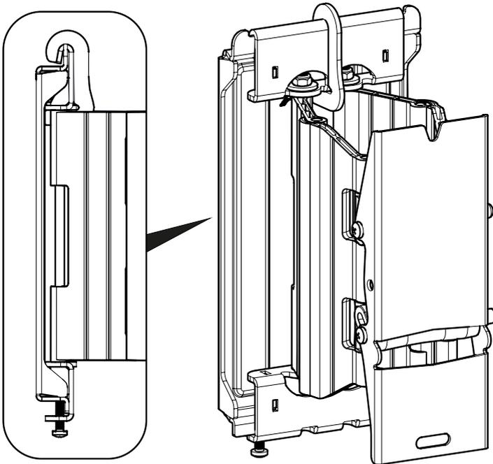
Tighten both screws to lock Mount Arm to Wall Plate.
