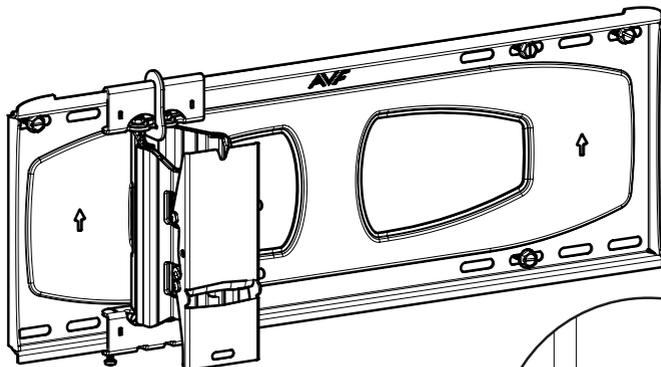
Slide arm into the required position and re-tighten both locking screws.
