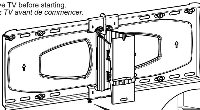
Loosen both locking screws.
