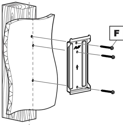
DO NOT use wall plugs in a wood stud wall.
