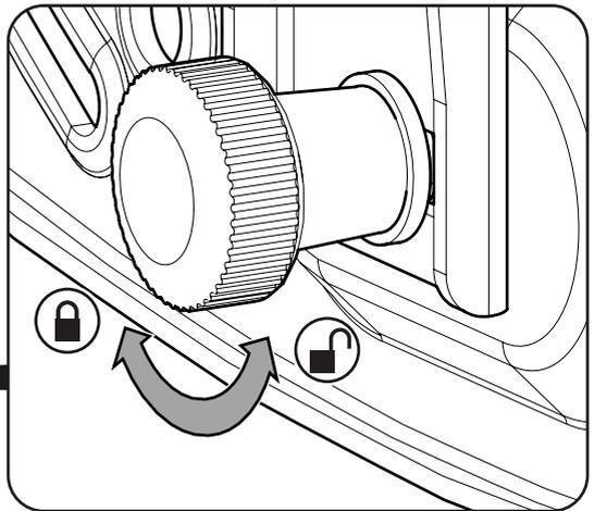
Loosen the Level Lock Screw, adjust your TV until it is level, then re-tighten the screw.
