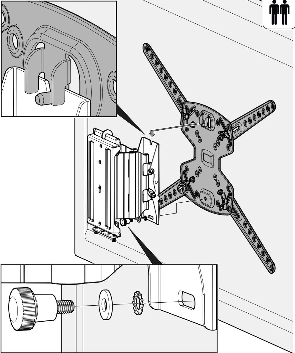
Reuse screw and washers saved in step 2. Make sure you fit the washers in the correct order.
