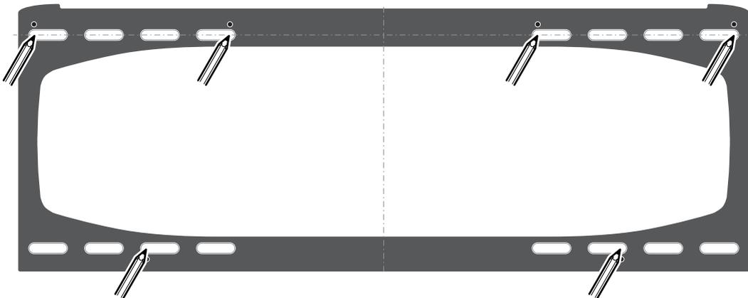
If fixing the Double Stud Wall Plate to a solid wall use the six fixing holes shown. If fixing to a wood stud wall only four screws are required. Position the Wall Plate so that it spans two wood studs and ensure each screw is in the centre of a wood stud.
