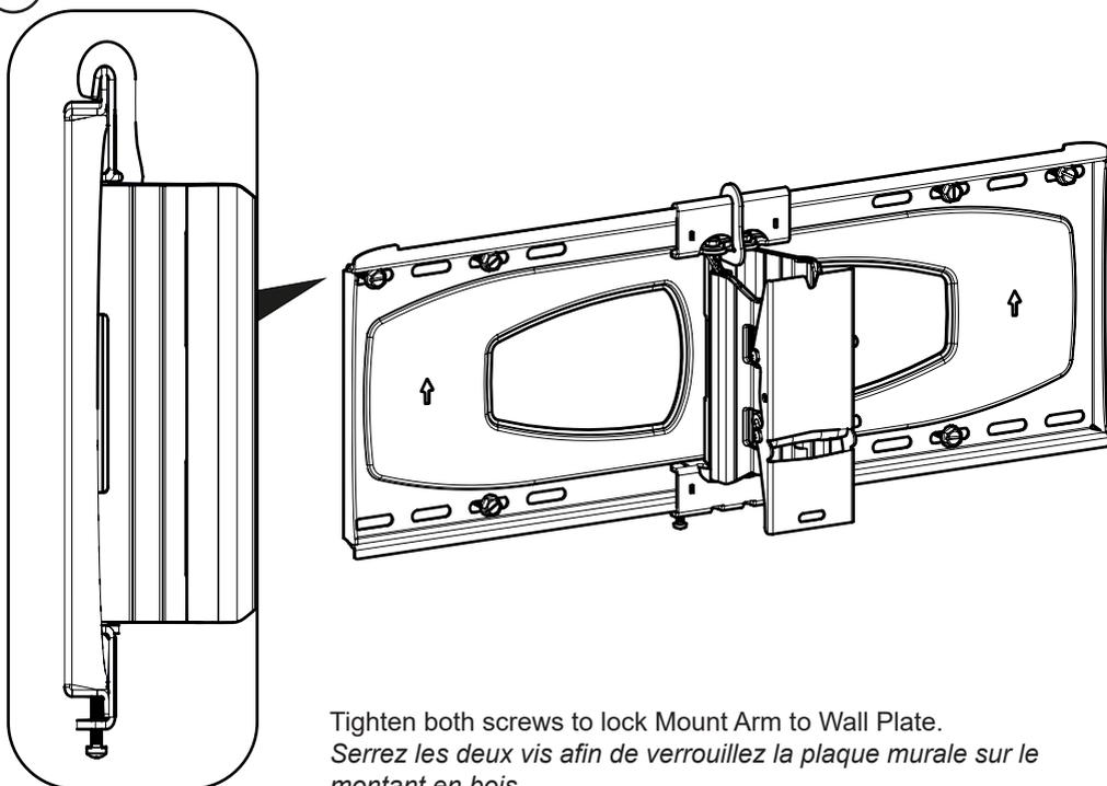
Tighten both screws to lock Mount Arm to Wall Plate.
