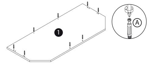
**NOTE**: Once part 1 is fitted secure with 8 part Bs. Make sure all part Bs are tightened to secure the top in place. Use Part D to cover any visible part B's.
