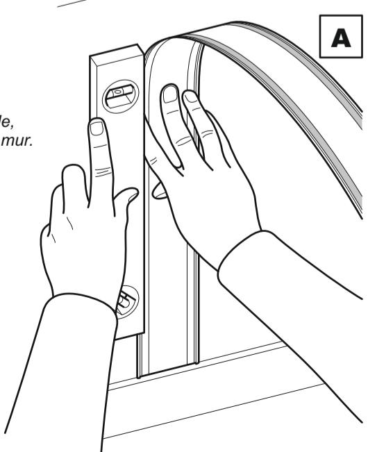
Using a spirit level as a guide, carefully stick wall strip **A** to the wall.
