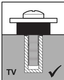
Attach the mounting plate to the back of your TV using suitable screw, reducer and spacer combinations.
