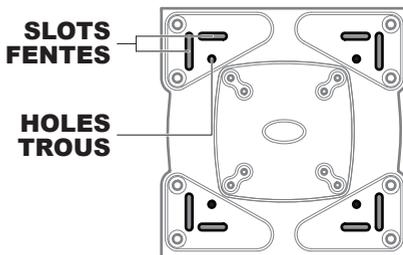
Before you fully tighten the TV mounting plate please check that the mounting plate holes line up with the fixing holes on the back of your TV.
