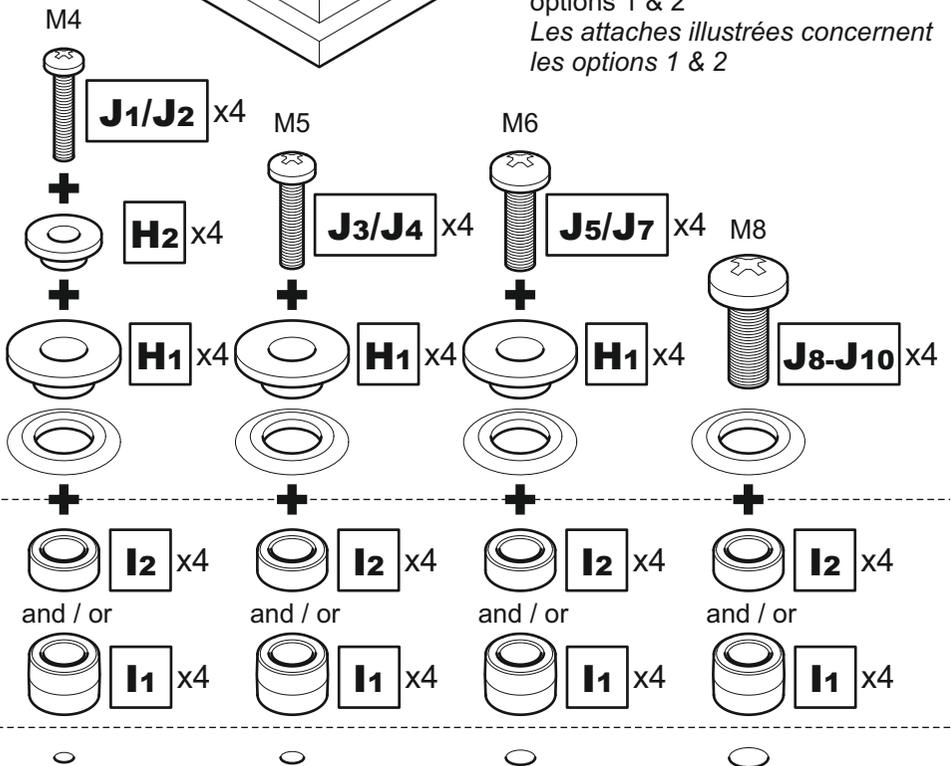
Attach the bracket to the back of your TV using suitable screw, reducer and spacer combinations.
