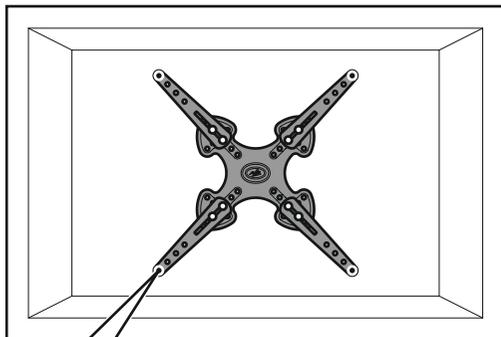
Holes line up and no adjustment is required before you fully tighten
