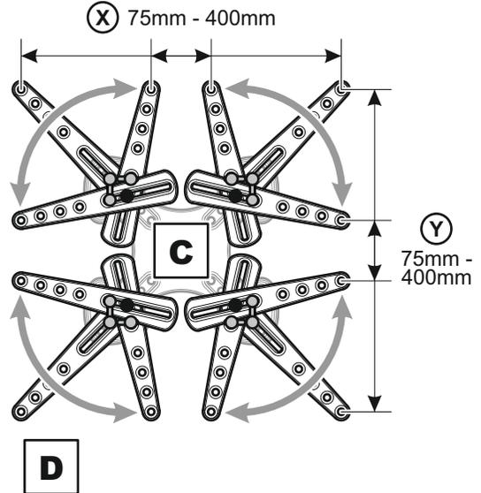
Adaptors **D** can be fixed in different positions in the slots on Plate **C** to match your TV fixing holes.
