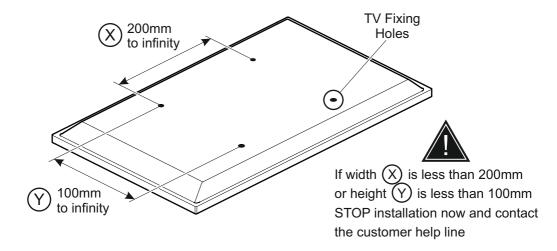
You are provided with 4 diameters of TV fixing screws, **M4**, **M5**, **M6** and **M8**. Determine the screw diameter that fits and remember for step 2.
