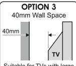
Suitable for TVs with large obstructions eg power supply, mouldings etc
