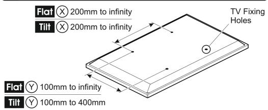
If width  $\bigcirc$  is less than 200mm or height  $\bigcirc$  is less than 100mm STOP installation now and contact the customer help line
