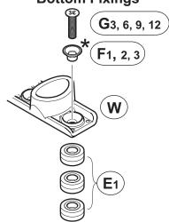
Use adapter (F<sub>1</sub>) with screws (G<sub>1</sub>), (G<sub>2</sub>) & (G<sub>3</sub>) Use adapter (F<sub>2</sub>) with screws (G<sub>4</sub>), (G<sub>5</sub>) & (G<sub>6</sub>) Use adapter (F<sub>3</sub>) with screws (G<sub>7</sub>), (G<sub>8</sub>) & (G<sub>9</sub>) No adapter required with screws (G<sub>10</sub>), (G<sub>11</sub>) & (G<sub>12</sub>)
