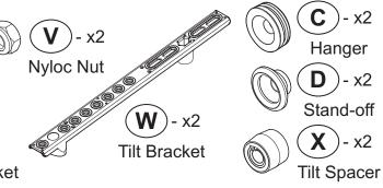
TV Fixings: Parts go on the back of the TV (specification of your TV will determine which ones you require - see section 11).
