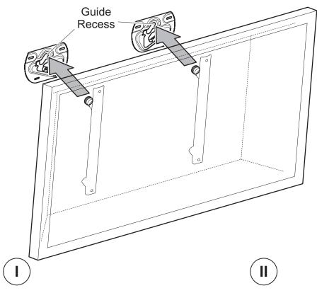
Present the Hangers (on the back of the TV) to the guide recess on the Wall Brackets. Slide down and across into place. Ensure both Hangers are fully engaged. If cables from the TV prevent the TV resting against the wall then an alternative hanger configuration will be required (See Section 20).
