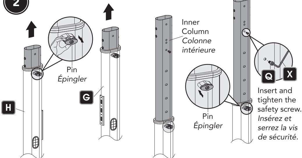
Pull the pin outwards and pull the inner column upwards at the same time, until the inner column is pulled to the desired height, then release the pin to secure.
