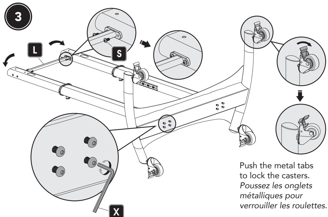
When the cross bar installation is complete, fully tighten the screws in the base.
