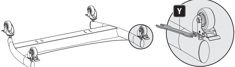
Each caster can be adjusted independently for fine tuning. Slightly turn the nut to lower or raise the base.
