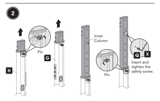
Pull the pin outwards and pull the inner column upwards at the same time, until the inner column is pulled to the desired height, then release the pin to secure.
