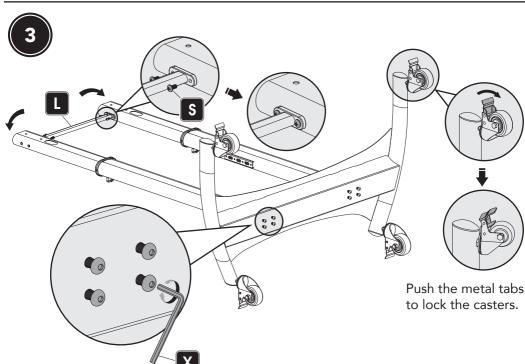
When the cross bar installation is complete, fully tighten the screws in the base.
