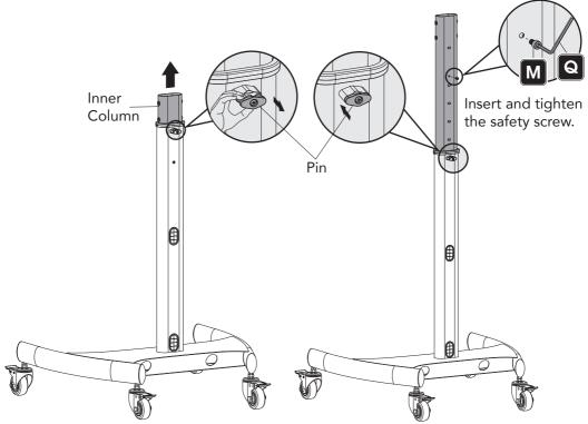
Pull the pin outwards and pull the inner column upwards at the same time, until the inner column is pulled to the desired height, then release the pin to secure.
