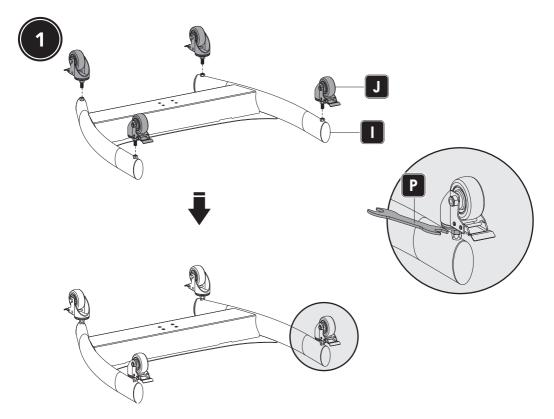
Each caster can be adjusted independently for fine tuning. Slightly turn the nut to lower or raise the base.
