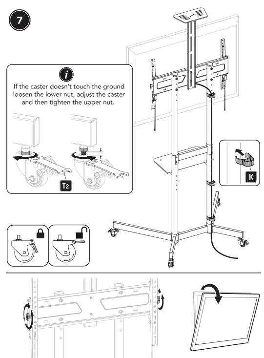
Loosen the knob to adjust the display to the desired angle. Tighten the knob to secure.
