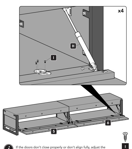
door hinge alignment screws small amounts until they do.
