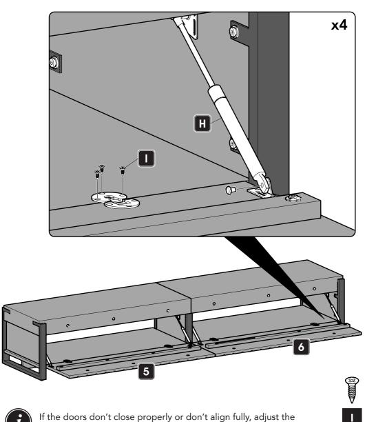
door hinge alignment screws small amounts until they do.
