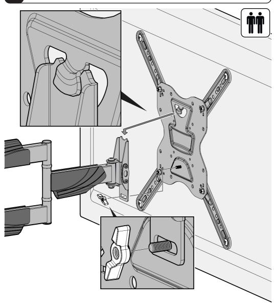
Reuse the Level Lock Thumb Nut saved in step 2.
