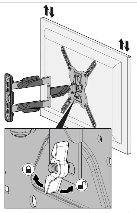
Loosen the Level Lock Thumb Nut, adjust your TV until it is level, then re-tighten the thumb nut.
