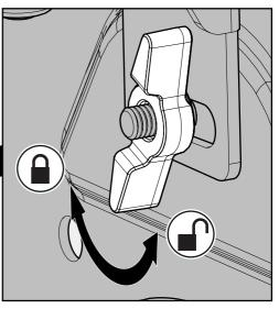
Loosen the Level Lock Thumb Nut, adjust your TV until it is level, then re-tighten the thumb nut.
