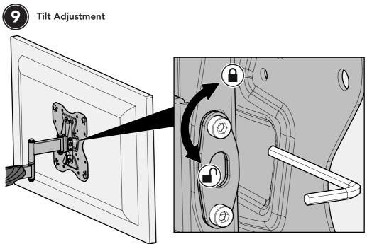
Adjust screws to achieve perfect tilt resistance if required. You must adjust both screws equally. You can also lock the tilt if required.
