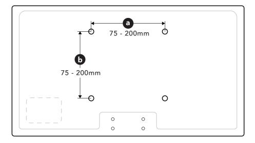
If width **a** is greater than 200mm or height **b** greater than 200mm STOP installation now and contact the customer helpline.
