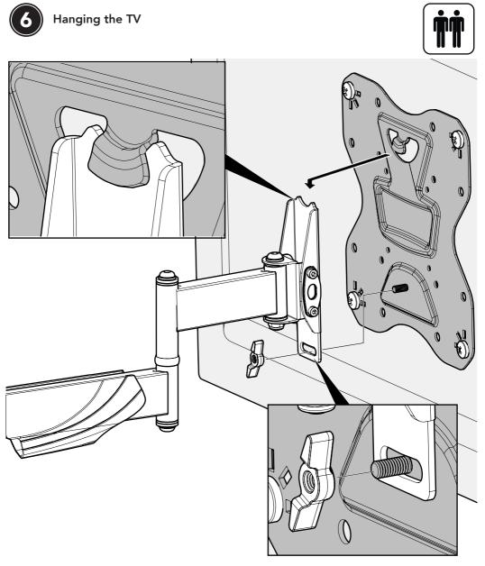
Reuse the Level Lock Thumb Nut saved in step 2.
