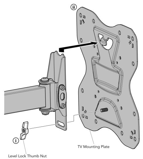
Remove the Level Lock Thumb Nut and safely keep for step 6.
