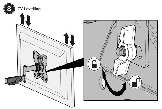
Loosen the Level Lock Thumb Nut, adjust your TV until it is level, then re-tighten the thumb nut.
