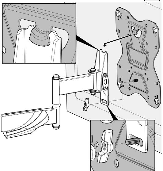
Reuse the Level Lock Thumb Nut saved in step 2.
