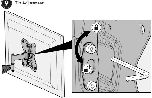
Adjust screws to achieve perfect tilt resistance if required. You must adjust both screws equally. You can also lock the tilt if required.
