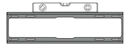
**ii** Make sure the TV brackets are level on the back of the TV. Adjust or re-fit if required.
