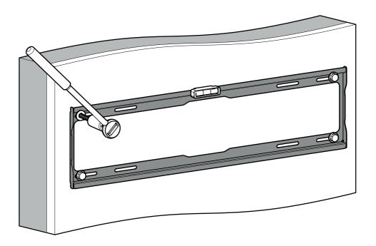
i Check the wall plate is perfectly level. Adjust or re-fit if required.
