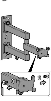
Remove the Screws and Washers and safely keep for step 4.
