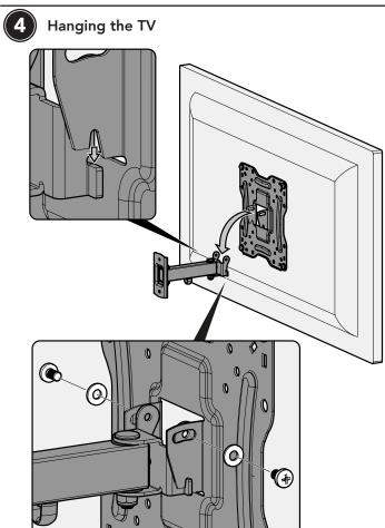
Reuse screws and washers saved in step 1.
