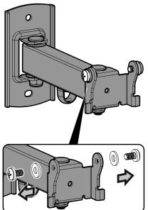
Remove the Screws and Washers and safely keep for step 4.
