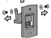
Remove the Screws and Washers and safely keep for step 4.
