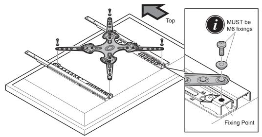
The brackets and screws etc shown in grey are only an example. These are supplied by the TV wall bracket manufacturer.
