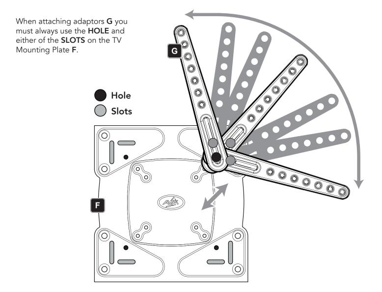
Adjust the adaptors **G** to fit the holes on the back of your TV. You can use any holes on the adaptors. The TV Mounting Plate must be level and vertically centered on the back of your TV.
