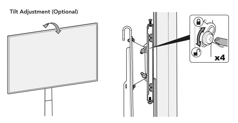
Adjust screws to achieve perfect tilt resistance if required. You can also lock the tilt if required.
