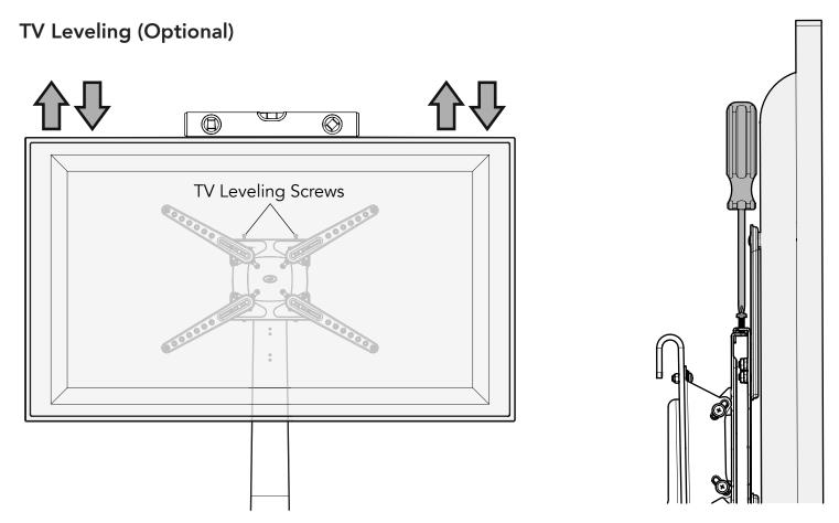
If your TV needs leveling, only adjust the TV Leveling Screw on the low side of the TV. For example, if the left hand side of your TV is low, adjust the left hand TV Leveling Screw only, until your TV is level.
