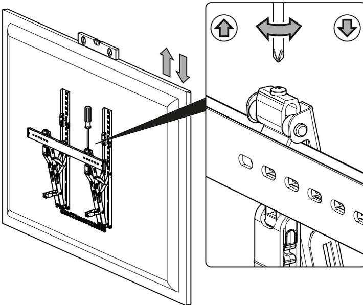
If your TV needs levelling, only adjust the TV Levelling Screw on the low side of the TV. For example, if the left hand side of your TV is low, adjust the left hand TV Levelling Screw only, until your TV is level.
