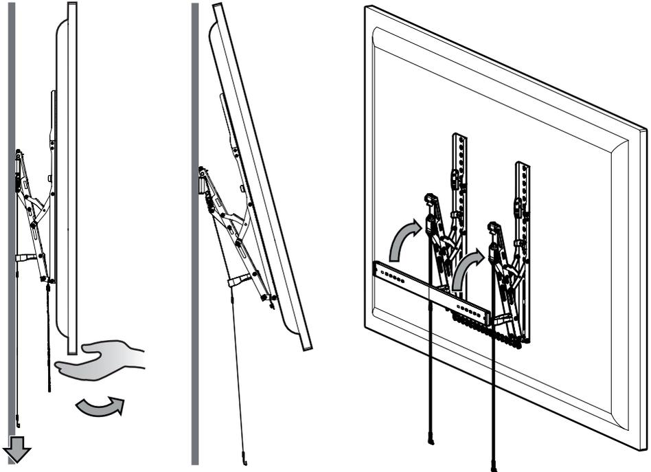
Pull both TV release cords at the same time to unlock the TV. Pull the bottom of the TV away from the wall so the catch cannot re-engage. Lift and remove the TV from the Wall Bracket.
