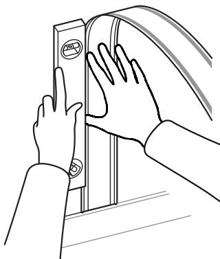
Use a clean, dry cloth to firmly press and rub along the channels.
