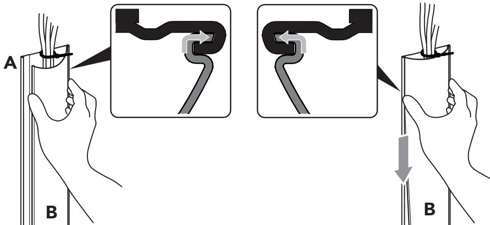
**TIP** To make it easier to keep cables in place while attaching Cover Strip **B**, you can wrap tape, or use a cable tie, around your cables at the top and bottom.
