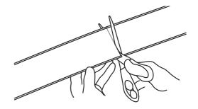
Remove backing paper from adhesive strips on Wall Strip **A**.
