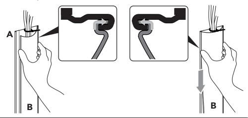
To make it easier to keep cables in place while attaching Cover Strip **B**, you can wrap tape, or use a cable tie, around your cables at the top and bottom.
