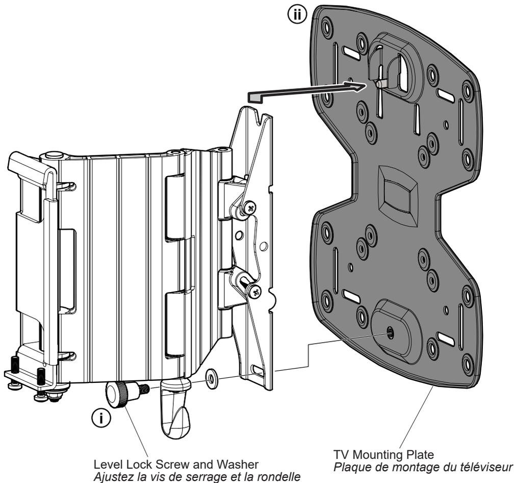
**i** Remove the Level Lock Screw and Washer and safely keep for step 10.
