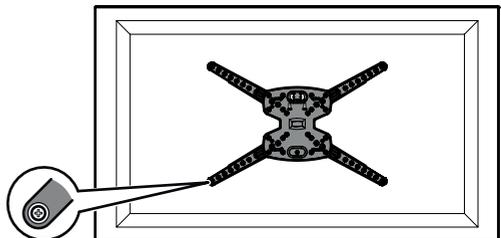
Holes line up and no adjustment is required before you fully tighten
