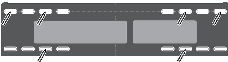
If fixing the Double Stud Wall Plate to a solid wall use the six fixing holes shown. If fixing to a wood stud wall you must place the Wall Plate so that it spans two wood studs. Ensure each screw is in the centre of each wood stud (only four screws required for wood stud installation).
