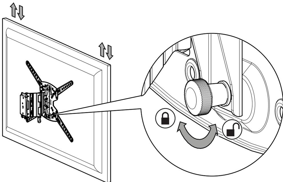
Loosen the Level Lock Screw, adjust your TV until it is level, then re-tighten the screw.
