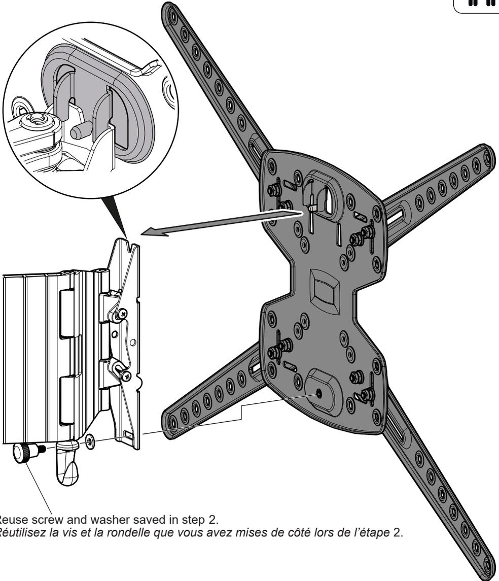
Reuse screw and washer saved in step 2.
