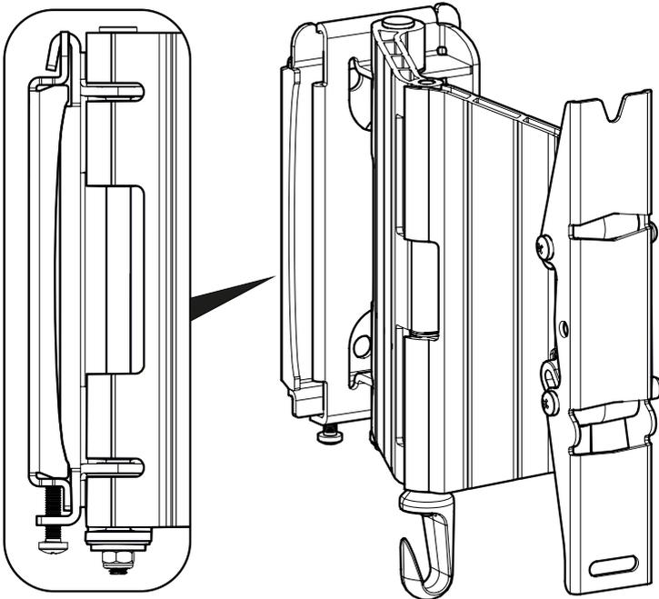
Tighten both screws to lock Mount Arm to Wall Plate.
