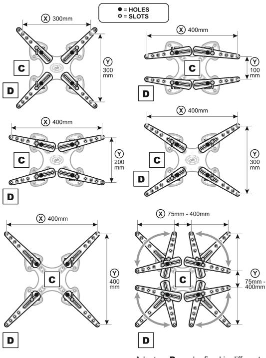
Adaptors **D** can be fixed in different positions in the slots on Plate **C** to match your TV fixing holes.
