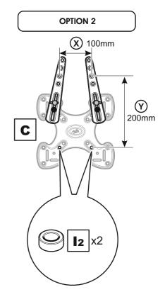
Use spacer **I2** between the bottom two holes of the bracket and your TV.
