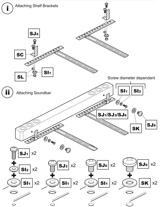
Attach the brackets to the back of your Soundbar using suitable screw and reducer combinations.
