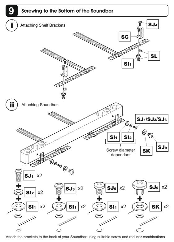
Please use this step in conjunction with the instructions provided with your TV wall mount. The brackets and the screws shown in grey are only an example. These are supplied by the TV wall mount manufacturer.
