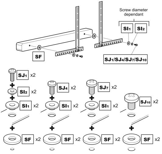
Attach the brackets to the back of your Soundbar using suitable screw and reducer combinations.
