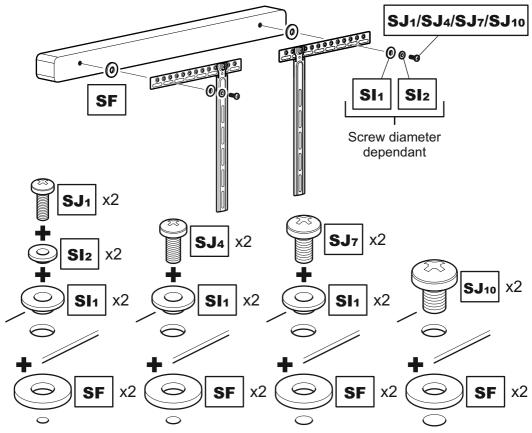
Attach the brackets to the back of your Soundbar using suitable screw and reducer combinations.
