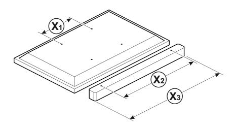
Measure the width of the fixing holes on the back of your TV (X1) and the back or bottom of your Soundbar (X2) or the length of your Soundbar (X3) if it has no fixing holes.
