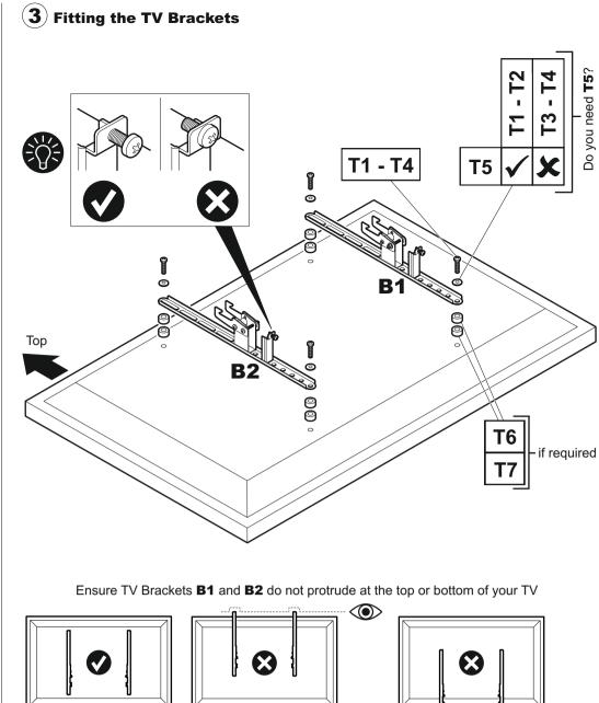
Attach the bracket to the back of your TV using a suitable combination of screw, washer
