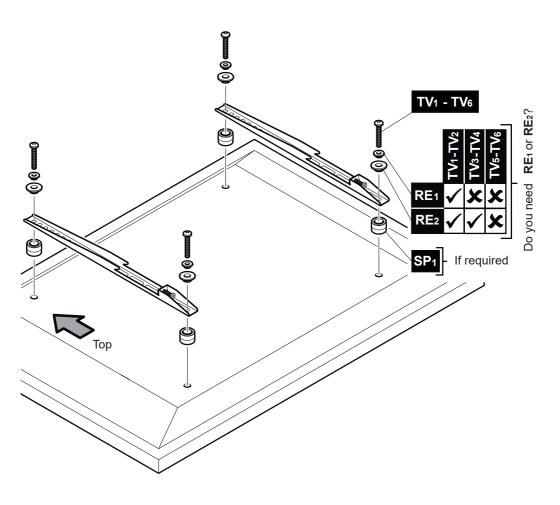
Attach the bracket to the back of your TV using suitable screw, reducer and spacer combinations.
