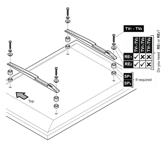
Attach the bracket to the back of your TV using suitable screw, reducer and spacer combinations.
