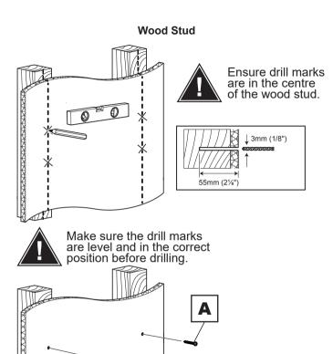
DO NOT overtighten screws. Tighten screws by hand only.
