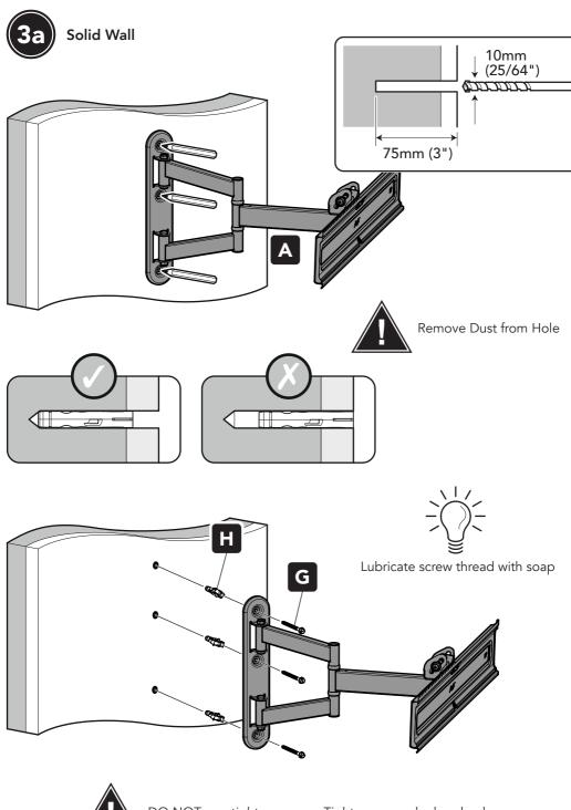
$\ensuremath{\mathsf{DO}}$  NOT overtighten screws. Tighten screws by hand only.
