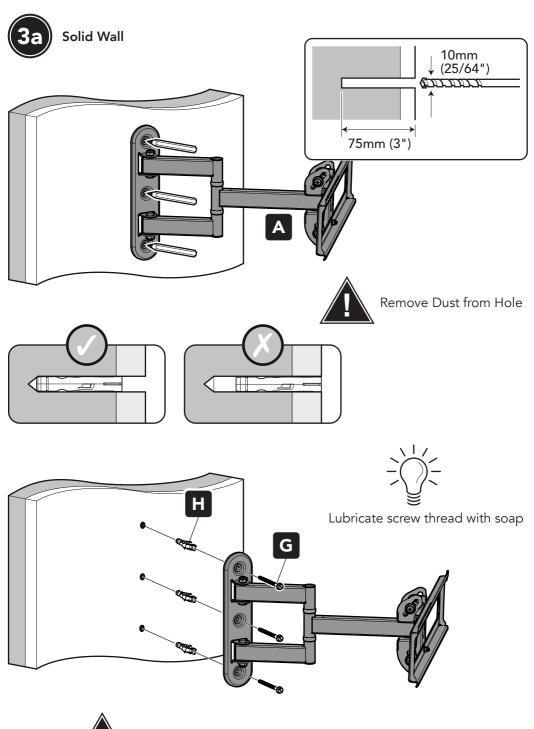
DO NOT overtighten screws. Tighten screws by hand only.
