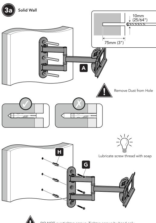
$\operatorname{DO}$  NOT overtighten screws. Tighten screws by hand only.
