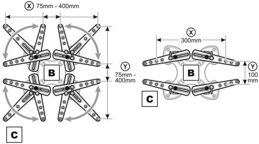
Adaptors **C** can be fixed in different positions in the slots on Plate **B** to match your TV fixing holes.
