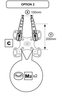
Use spacer **M2** between the bottom two holes of the bracket and your TV.
