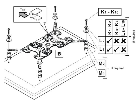
Attach the bracket to the back of your TV using suitable screw, reducer and spacer combinations.
