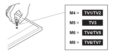
You are provided with 4 diameters of TV fixing screws, **M4**, **M5**, **M6** and **M8**. Determine the screw diameter that fits and remember for step 9.
