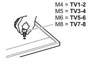
You are provided with 4 diameters of TV fixing screws, **M4**, **M5**, **M6** and **M8**. Determine the screw diameter that fits and remember for step 10.
