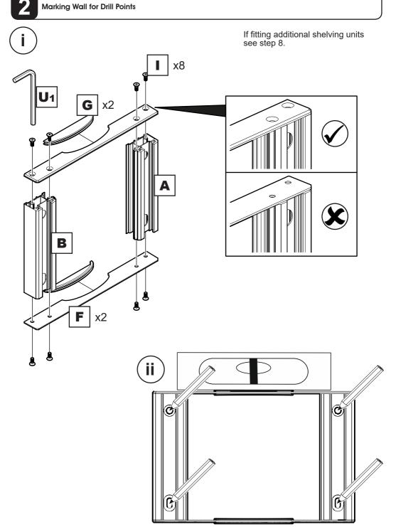
Use the correct fixings for your wall type. Mixing fixing types may be required for installations that span different wall types. DO NOT OVER TIGHTEN SCREWS.
