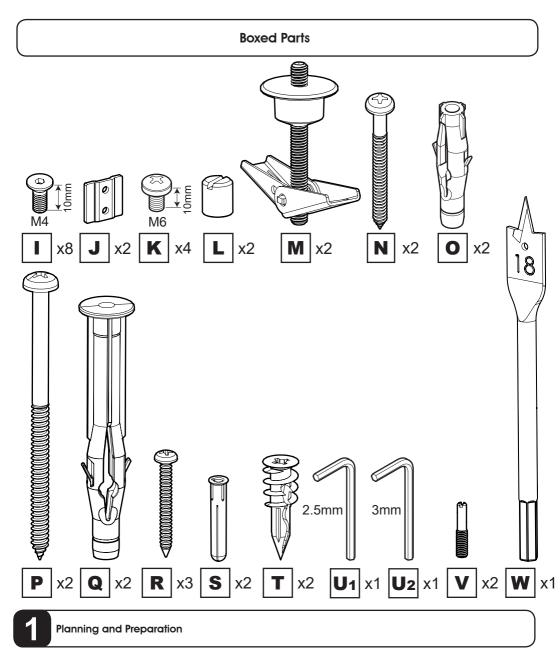
Determine the wall type that you have (i.e. Brick/Stud/Plasterboard/Sheetrock). Ensure the drilling area is free from mains services (Gas/Electric/Water). Drill three 3mm pilot holes to verify the wall type and select the appropriate fixings.
