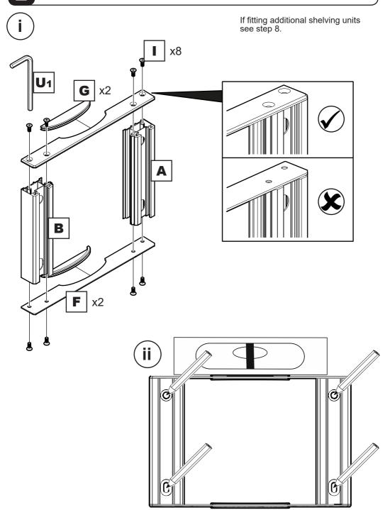
Use the correct fixings for your wall type. Mixing fixing types may be required for installations that span different wall types. DO NOT OVER TIGHTEN SCREWS.
