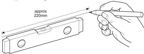
Use the Wall Bracket (A) as a template and position it on your wall. Ensure the bracket lines up with the line you have previously drawn and mark the two DRILL POINTS with a pencil.
