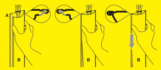
To make it easier to keep cables in place while attaching Cover Strip B, you can tie a small string or cable tie around your cables at the top and bottom.
