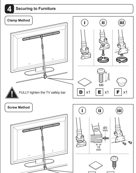
FULLY tighten the TV safety bar A
