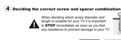
You are provided with 4 diameters of TV fixing screws, **M4**, **M5**, **M6** and **M8**. Determine the screw diameter that fits and remember for the next step
