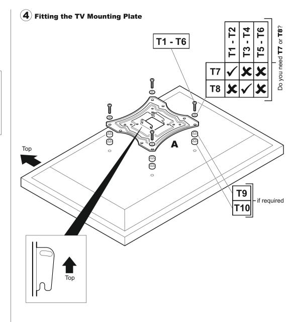
Attach the bracket to the back of your TV using a suitable combination of screw, washer and spacer combinations. **DO NOT OVERTIGHTEN!**
