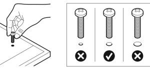
Spacers are provided so that you can achieve the correct fit between the back of your TV and Mounting Plate, please see below for examples of when spacers are required
